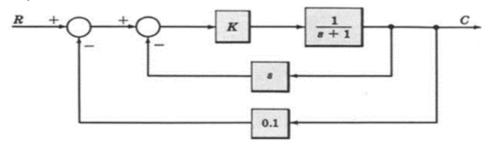
3) Find the close loop transfer function and characteristics equation of the given system.
