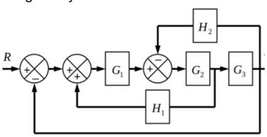
4) Construct the signal flow diagram, for the equation given in the figure. K2 (6)
