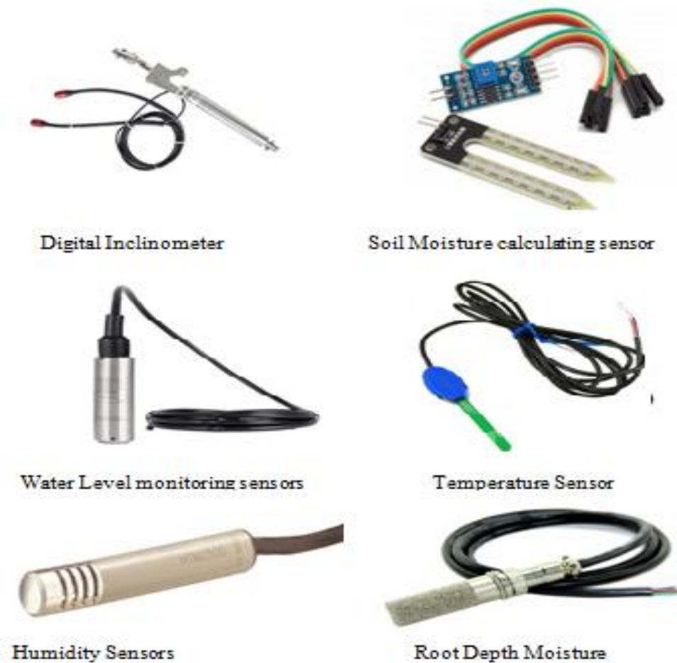
Figure 1.2: IoT Components of Irrigation System
