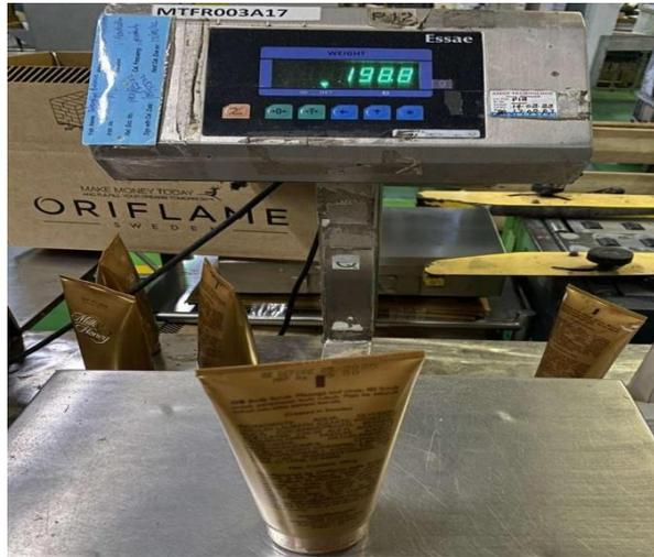
**Fig. 18: Checking weight during finish good inspection**
