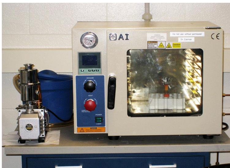
**Fig. 19: Vacuum Oven for leakage testing**
