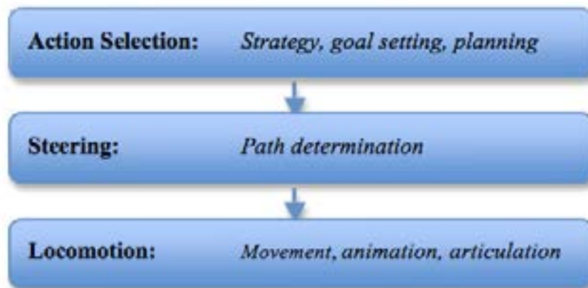
Figure 6.6 The hierarchy of motion behaviours used for the Boids model (Reynolds, 1987).
