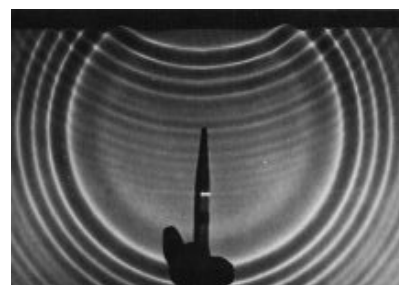
b / Circular water waves are reflected from a boundary on the left.
