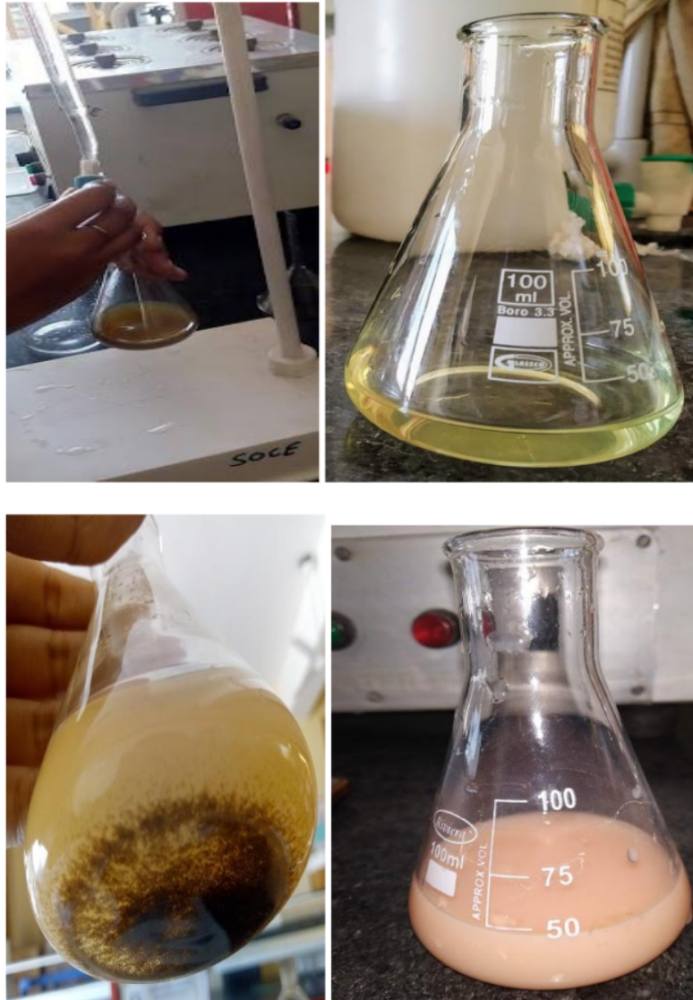
Figure 18: Determination of Chloride Content
