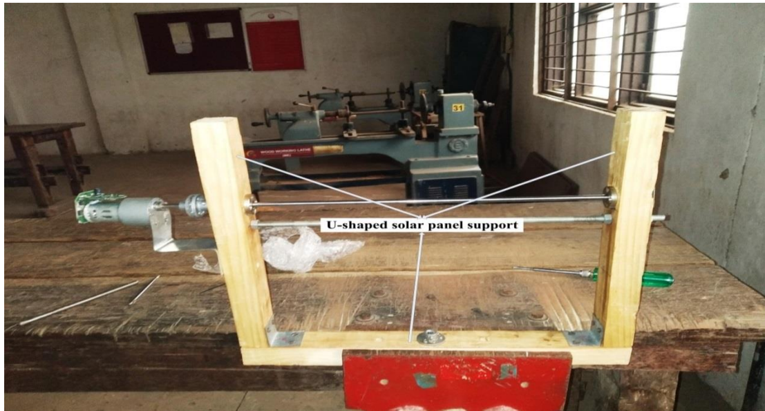
Figure 3.2 U-shaped solar panel supports
