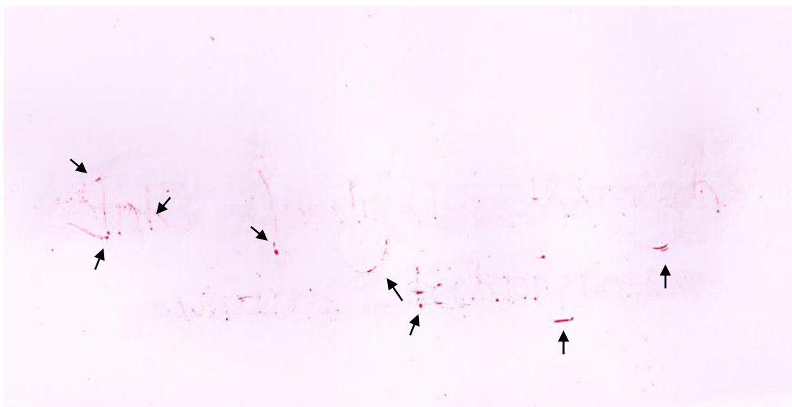
Figure 3.24: Few traces at the end of strokes reappeared when Pilot RED pen writings on the glossy paper is removed by using friction (rubber erasure)
