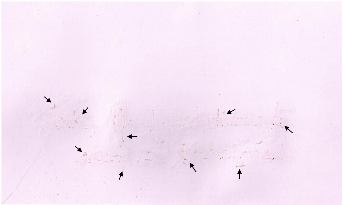
Figure 3.23: Few traces at the end of strokes reappeared when Pilot BLACK pen writings on the glossy paper is removed by using friction (rubber erasure)
