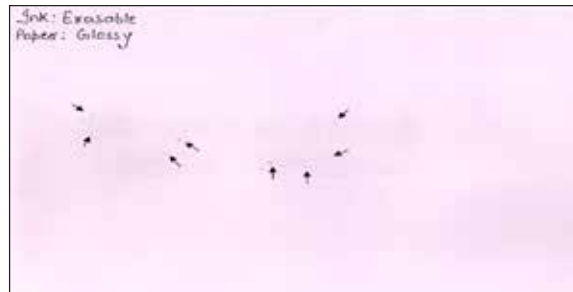
Figure 5: Few traces at the end of strokes reappeared when writings on the glossy paper is removed by using friction (rubber erasure)
