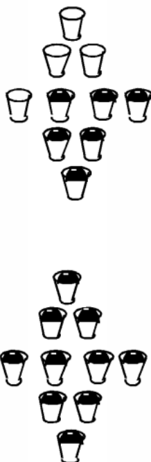
Figure 1.9: Electron distribution for a metal or good conductor
