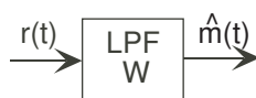
Figure 6.5: The receiver for baseband communication systems is quite simple: a lowpass filter having the same bandwidth as the signal.
